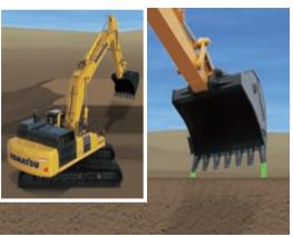
Minimum distance control The intelligent Machine Control excavator controls the bucket by automatically selecting the point on the bucket closest to the target surface. Should the machine not be facing a sloped surface at a right angle, it will still follow the target surface and minimize digging below it.
