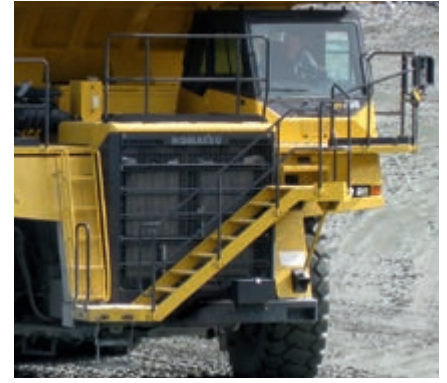
Safe cab access The low angle of the front stairways with handrails, slip-resistant
